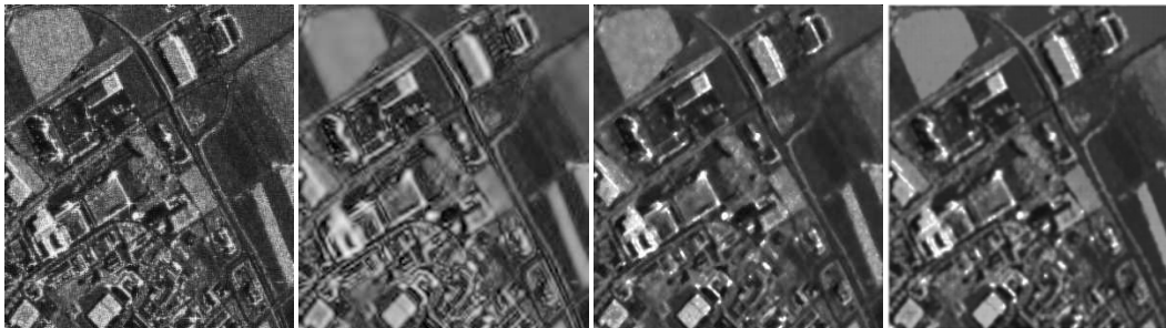
Figure 9: Results for the SAR Image III : (Left to right) The SRAD filter, the MAP-LG filter, the EBNL filter and the O -EBNL filter for \mathbf{z} = [18.72, 0.85, 0.87, 0.72, 7, 1, 5 \times 5, 9 \times 9]
